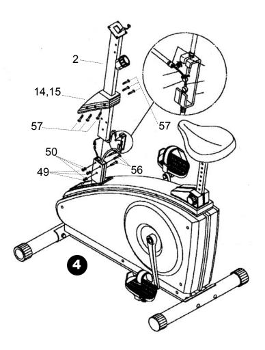
**4.** Slide the console tube (2) through the console tube collar (14, 15). Connect the computer cable in the console tube to the computer cable in the main frame. Connect the tension cable in the console tube to the tension cable connection in the main frame. Attach the console tube (2) to the frame with the locknuts (49), flat washers (50) and screws (56) provided. Attach the console tube collar (14, 15) to the main frame (1) with screws (57).
